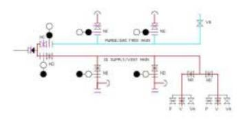
Figure 2 - FPSO cargo tank venting through IG Vent main and risers P+S. IG Supply/Vent main contains HC, Purge/Gas free main contains air.
