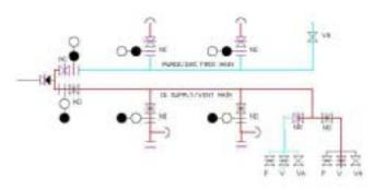
Figure 9 - Riser valves overhaul. IG Supply/Vent main contains HC, Purge/Gas free main contains air.
