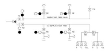
Figure 1 - FPSO basic layout IG deck pipe distribution system
