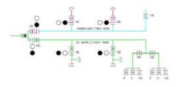
Figure 3 - FPSO - cargo tank IG topping up while discharging via IG Supply main.
