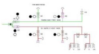
Figure 4 - FPSO cargo tank purging with IG supply via Purge main and venting P+S via Vent main. IG Supply/Vent main contains HC, Purge/Gas free main contains IG.
