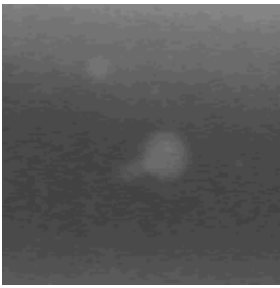
Figure 3.13 Gray scale image of Figure 3.12 (X-ray Image of Defect in a Pipe Weld)
