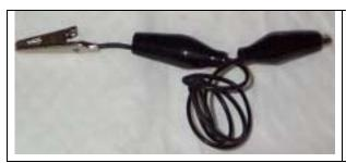
This is a wire clip. It's nothing more than a length of wire with two alligator clips on the ends. The clips have a plastic cover over them to prevent them from touching wires or components that they are not clipped onto.
