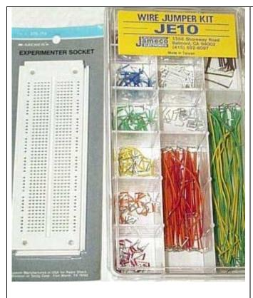
Breadboard and wire jumpers are an experimenter's best friends! The breadboard is a solder less socket board. This is the \$11 version from Radio Shack, though I want to point out you can buy cheaper ones from <u>Jameco</u> and <u>B&G Micro</u>.
