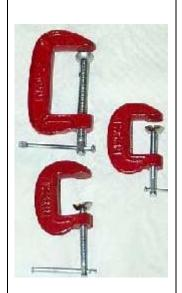
Something else very good for holding things is a clamp. You can use clamps for a variety of different jobs, such as holding wood down to a table while you are cutting it. Holding wood or plastic together and in straight alignment for drilling.
