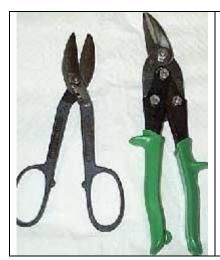
Our next tools are both tin snips. These are used for cutting aluminum sheeting. Aluminum sheeting is a cheap way to give your robot that all metal look when in fact that frame underneath is all light weight wood.
