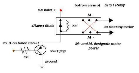
The next circuit is the DPDT motor driver. If you built the first one with out a problem you should have no problem with this one. Note: that N.C. and N.O. pins on the relay are crossed. This flipflops the power so as to reverse the power to the drive motor. Again you can test this circuit the same way as the power circuit.
