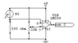
This is the light sensor. It sends a signal to the power circuit. Adjust the 10K pot so Bolo-Bot knows when he is hidden and when he is not. On the robot you will want to place the light sensor on the top of Bolo-Bot. You may want to put a tube around the sensor to limit its sensor range. You would want this if it runs under a table so it does not pick up ambient light, which would confuse the sensor.
