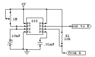
This is the last circuit of Bolo-Bot. This is a timer that is triggered by the bump sensor. The bump sensor attaches at point A. When Bolo-Bot bumps into something the timer shuts off for a second or two then come back on. When this happens the DPDT relay reverses the drive motor until the timer comes back on. This allows Bolo-Bot enough time to turn around and head in a new direction. Timers are tricky! You may have to play with the 1M pot to get the right amount of time for your robot.
