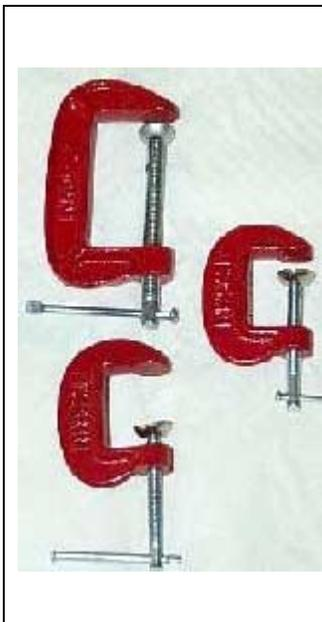
Something else very good for holding things is a clamp. You can use clamps for a variety of different jobs, such as holding wood down to a table while you are cutting it. Holding wood or plastic together and in straight alignment for drilling.
