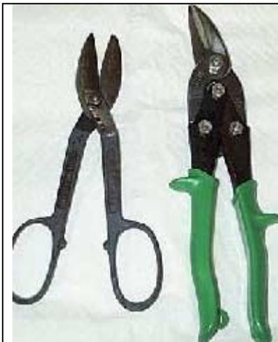
Our next tools are both tin snips. These are used for cutting aluminum sheeting. Aluminum sheeting is a cheap way to give your robot that all metal look when in fact that frame underneath is all light weight wood.
