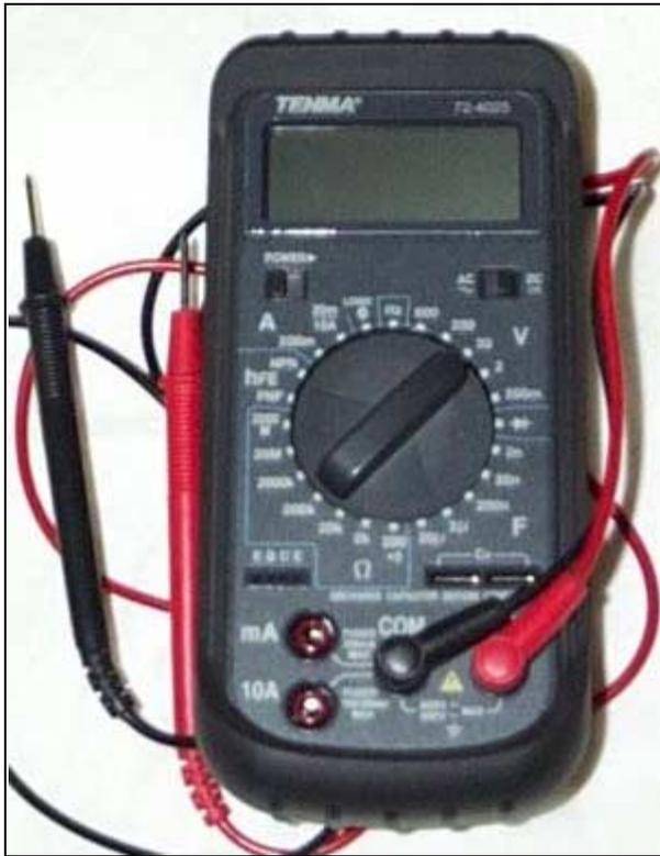
Now we get to the mother of all electronics tools, the Multimeter! Multimeter live up to their name, they allow you to monitor multiple electronics readings with one tool.
