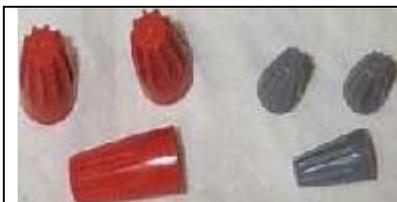
Our next item is wire nuts. Wires nuts are used to cap off and connect wires that have been twisted together by hand. This is much better than using electrical tape to cover the bare ends of connected wires. Wires nuts come in all different sizes, bigger nuts are for thicker wires.
