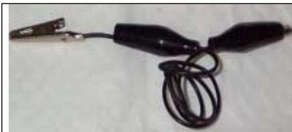
This is a wire clip. It's nothing more than a length of wire with two alligator clips on the ends. The clips have a plastic cover over them to prevent them from touching wires or components that they are not clipped onto.
