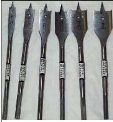
How do you make a hole? The answer is with big drill bits! This is a set of hole making drill bits from 3/8" of an inch up to 1" inch wide. You can use them to make holes in wood or plastic.
