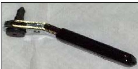
This is a ratcheting screwdriver. You can stick in any normal screwdriver bit into this ratchet and in fact this Craftsman tool comes with a set of driver bits. Cost was \$10 from Sears and was well worth it. I have not seen another tool like it and it fits into the smallest places. It really comes in handy when you have a small case for protecting your robot's controller and you need to drive a screw from the inside of the case.
