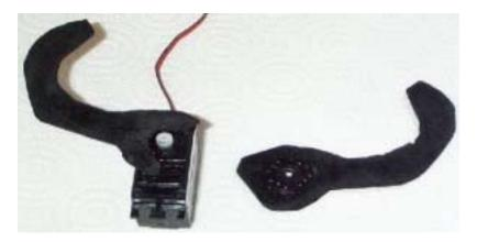
The stationary finger is glued onto the servo case in a permanent position. This finger is positioned so that when the moving finger is in an open position, the gripper has the best possible opportunity to grasp something. Notice that the finger on the case has a hole big enough so that it does not interfere with the way the servo horn connects to the servo.
