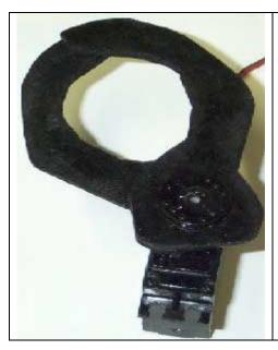
To the left is a picture of the gripper closed, which better show what the gripper looks like and how it will function once complete. The top finger (the one controlled by the servo) closes just slightly over the bottom stationary finger.
